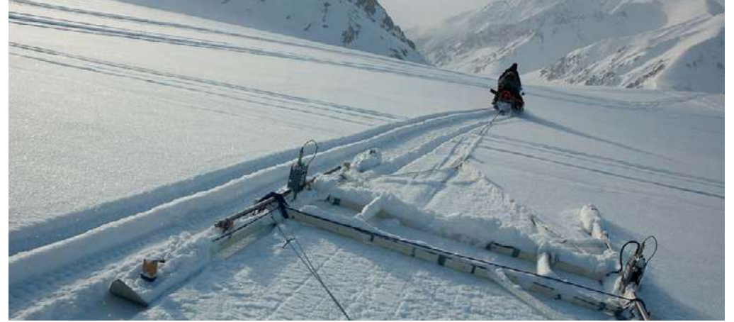
Measuring the ice thickness of a glacier in Greenland by ground penetrating radar Credit: G. Weyss
