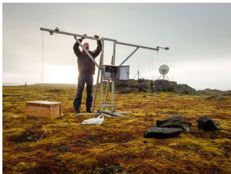
Installation of solarphotometer by Estonian scientist at Polish station Hornsund on Svalbard. Photo: Timo Palo
