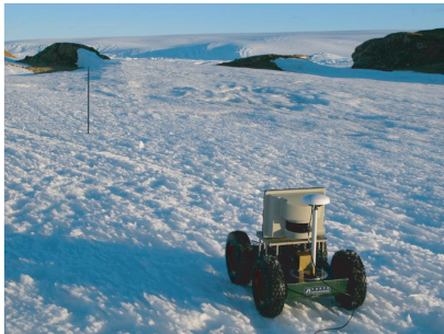
Fig. 5 The simulated experiment of glacier movement observation.
