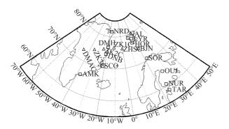
**Figure 2** Chinese Antarctic Magnetometer (CAM) chain conjugated regions in the Arctic. The CAM chain comprises five sites, i.e., ZHS, ZK1, ZK2, ZK3 and DMA, conjugated with ZHSC, ZK1C, ZK2C, ZK3C and DMAC, respectively. Plotted together are several magnetometer sites in the Arctic region, such as NAL from the IMAGE chain and DMH from the East Coast chain of Greenland Island. The coordinate labels are in geographical (GEO) system.
