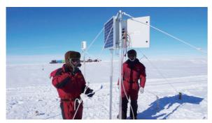
**Figure 4** A low power magnetometer (LPM) running in inner land of Antarctica, which consists in a sensor, a data recording box, a set of storage battery, a solar panel and a wind generator. The sensor and the storage battery are buried under the ice/snow, while the data recording box, solar panel and the wind generator are supported by aluminum poles above the ground.
