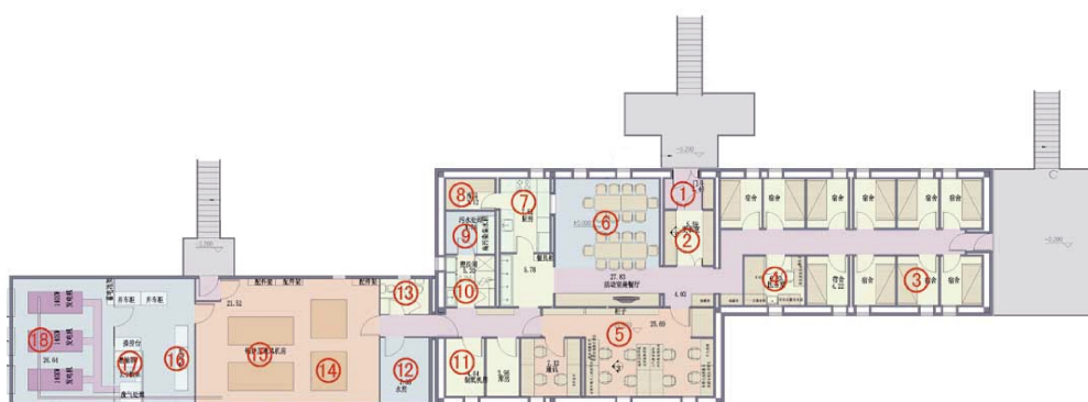
Figure 11 Plan of the main building: (1) foyer, (2) changing room, (3) sleeping area, (4) clinic, (5) scientific research room, (6) activity room, (7) kitchen, (8) warehouse, (9) sewage treatment, (10) bathroom and laundry, (11) oxygen equipment, (12) water supply, (13) bathroom, (14) ventilation equipment room, (15) boiler room, (16) distribution and control room, (17) temporary storage, and (18) generator room.
