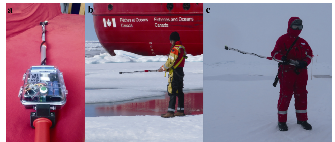
Figure 1 a, Photo of the completely assembled albedo wand; b, Albedo wand used to measure the albedo of a melt pond during the Amundsen 2018 expedition in Baffin Bay, July 2018; c, Albedo wand used in harsh Arctic autumn climate close to the geographic North Pole during the Oden expedition, September 2018.
