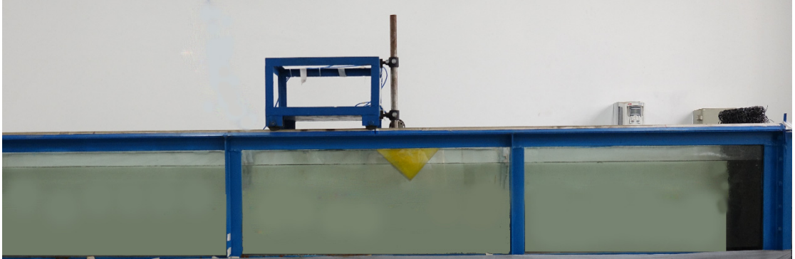
Figure 1 Photograph of laboratory wave tank with ridge-keel model (in yellow).
