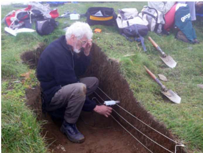
Magnetic susceptibility measurement on solifluction lobe Paltina (Făgăraș Mountains). (Photograph provided by Petru Urdea).
