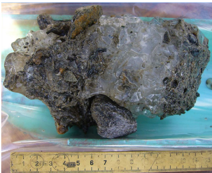
Ice encountered during the Lazaun rockglacier drilling (Val Senales, Alto Adige) (Photograph provided by K. Lang)
