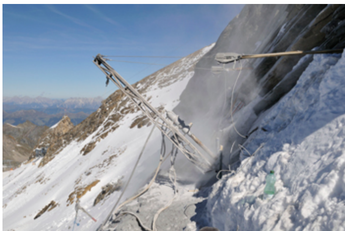
Air flush rotary drilling of a 30m deep borehole at the Kitzsteinhorn, Hohe Tauern Range, during early autumn 2011 at about 3000 m a.s.l. Photograph provided by Ingo Hartmeyer.
