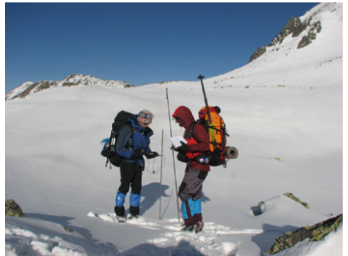
Fig. 6. Monitoring of annual ground surface temperature using miniature temperature data loggers and bottom temperature of snow measurements on periglacial landforms of rock glaciers and talus slopes from Retezat (Photo P. Urdea).
