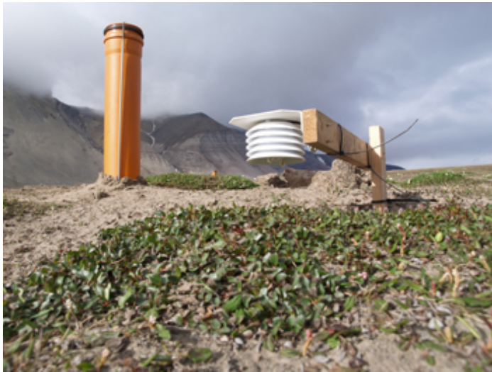
Fig. 5 – Ground temperature and humidity measurements devices in Ebba Valley on the vegetation growth plot (photo by A. Buchwal)
