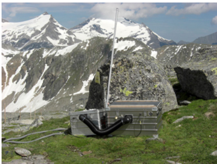
Permanent geoelectric monitoring profile installed between October 2010 and July 2011 in the vicinity of Mölltaler Glacier at 2760 m a.s.l. The used instrument GEOMON4D is a continuous, stand alone, DC resistivity monitoring instrument developed by the Geological Survey of Austria. Photograph provided by Birgit Jochum.
