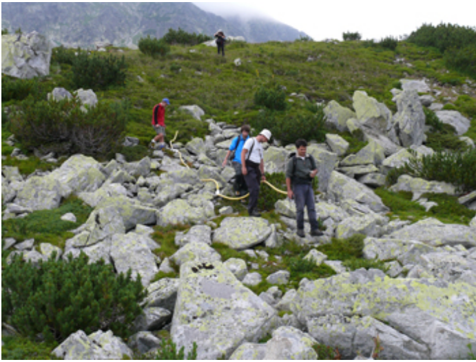
Fig. 1. GPR investigations in Ana rock glaciers, Retezat Mts. Fig. 4. (Photo, P. Urdea).
