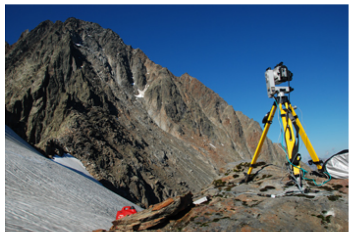
Terrestrial laserscanner at Ritzlihorn (Bernese Alps), summer 2010, after a large debris flow damaged infrastructure in the underlying valley (Photo: M. Philipps).
