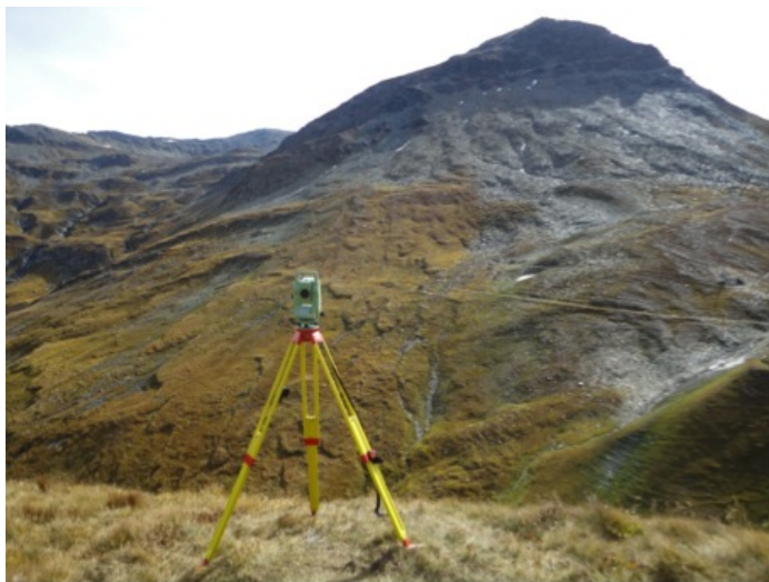
Figure 2. Terrestrial geodetic survey of solifluction lobes on the north slope of Blaubeerg, Furka (Photo: A. Rist).
