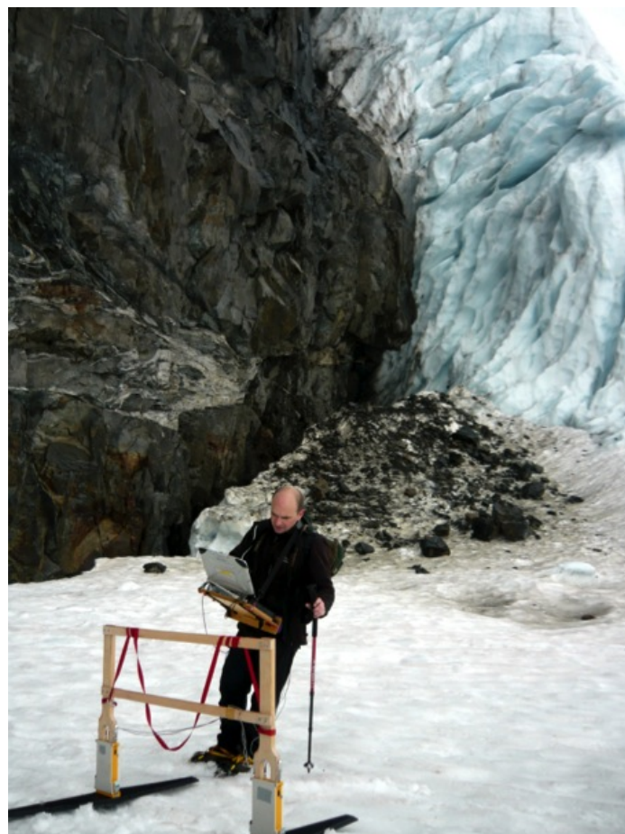
Figure 3. GPR measurements on Storglaciaren, Kebnekaise, northern Sweden, (Photo by W. Dobiński)
