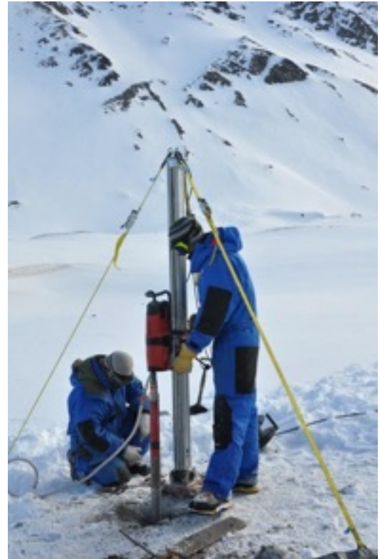
Figure 1. Drilling of piezometers in the proglacial area of Austre Lovén glacier close to Ny-Ålesund- Svalbard (April 2013). The piezometers are equipped with CTD probes and temperature loggers (0.5 to 4.5 m deep) – photos taken by Christelle Marlin.
