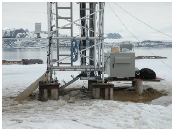
Figure 2. Eddy covariance flux system at a height of 22 m (LHS) and Cavity Ring-down Spectrometer (closed-path gas analyzer) in the cabinet (RHS) at Amundsen-Nobile Climate Change Tower
