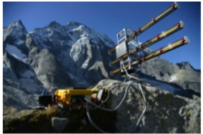
Figure 5. Interferometric radar measurements by A. Kos at Pizzo Cengalo on 13.9.2013 (Photo: M. Phillips).
