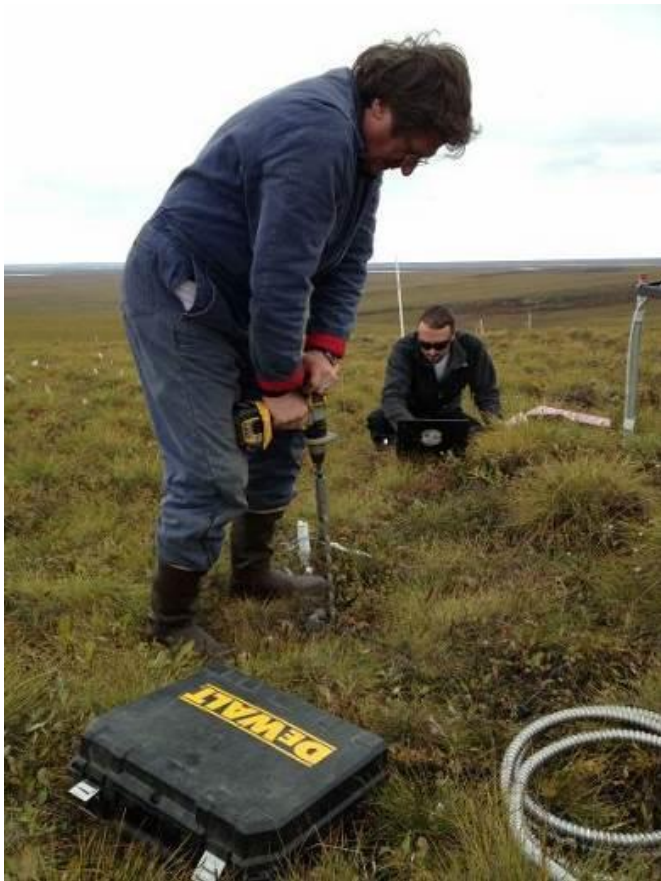
Figure 4. Vladimir Romanovsky (GIPL Group Leader) drilling a hole in the ground to install temperature sensors and Bill Cable preparing the sensors for installation at a permafrost observation station on North Slope of Alaska (Photo: Santosh Panda).
