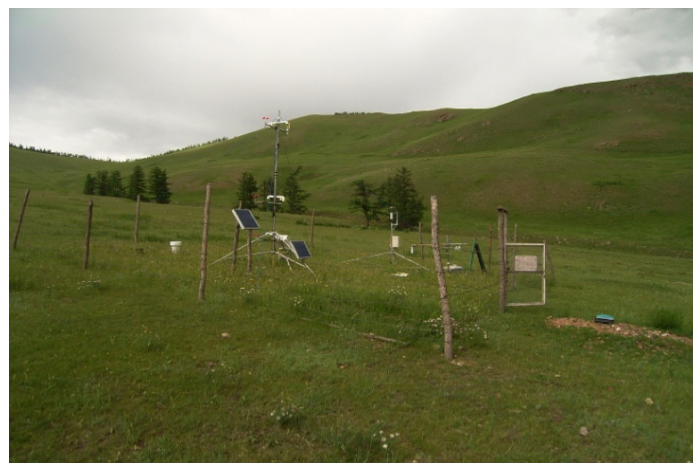
Figure 1. AWS at the observation site-Terelj J site (photo by Dr Y. Iijima)
