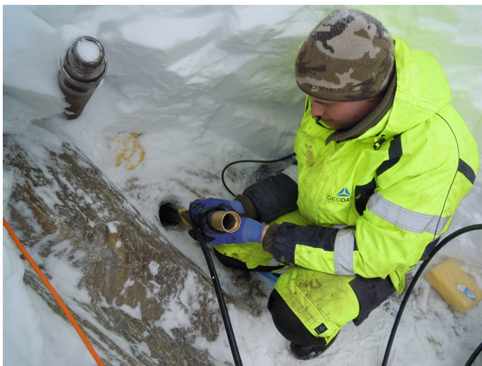
Figure 2. Borehole in permafrost-affected rock which is instrumented with a protective casing, Kitzsteinhorn, Hohe Tauern Range, at an elevation of 3030 m a.s.l. Photograph provided by Ingo Hartmeyer.
