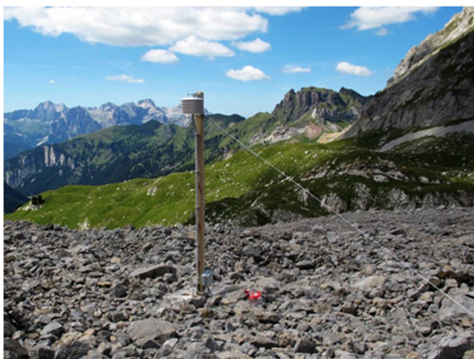
Figure 2. The station for measuring air temperature, snow cover thickness and ground surface temperature installed on the Cima Uomo rock glacier (Dolomites, Eastern Italian Alps).
